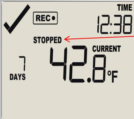
When it is time to download the data from the data logger we suggest stopping the logger. To accomplish this you hold down the Start/Clear/Stop button for 1-2 seconds. The word STOPPED will appear on the screen as shown on the top left picture. The REC symbol will disappear after 1-2 seconds and you take your finger off the button quickly.
