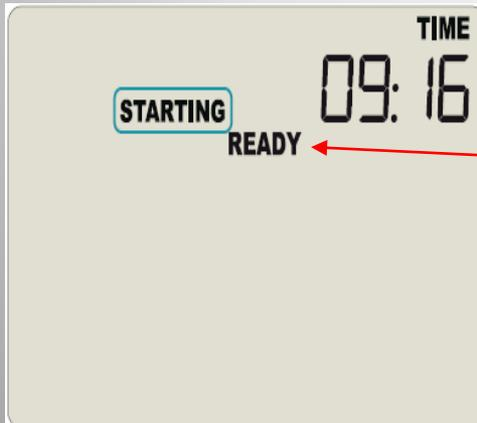
To Start: Press and hold the Start/Clear/Stop button. First, STARTING is displayed in addition to READY. Then READY disappears.
