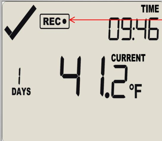
Once READY disappears, immediately release the button. STARTING will also disappear, and the symbol REC• will be shown. The VFC 400 is now recording temperature data.
